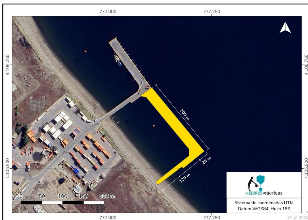
Figure 3-6: Extension of the pier
